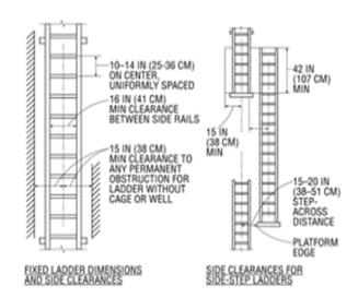
Figure D-2 -- Side-Step Fixed Ladder Sections
