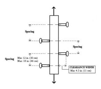
Figure D-6 -- Step Bolt Spacing
