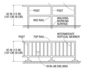
Figure D-11 – Guard Rail Systems
