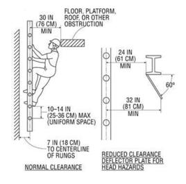
Figure D-5 -- Fixed Ladder Clearances
