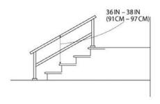
Figure D-13 – Combination Handrail and Stair Rail
