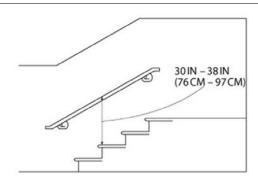
Figure D-12 – Handrail Measurement
