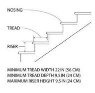
Figure D-8 – Dimensions of Standard Stairs
