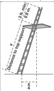
Figure D-1 -- Portable Ladder Set-up
