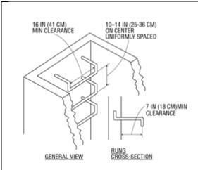
Figure D-4 -- Individual Rung Ladder
