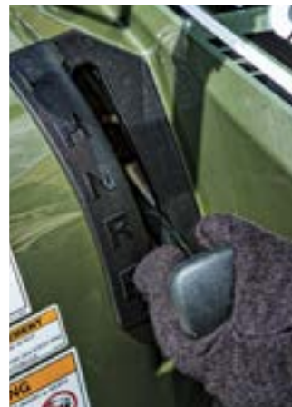
On-the-fly 2WD/4WD with front differential lock
