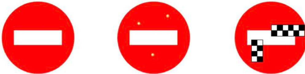
Figure 6. Traffic sign images: normal with pixel errors and with injected fault.
