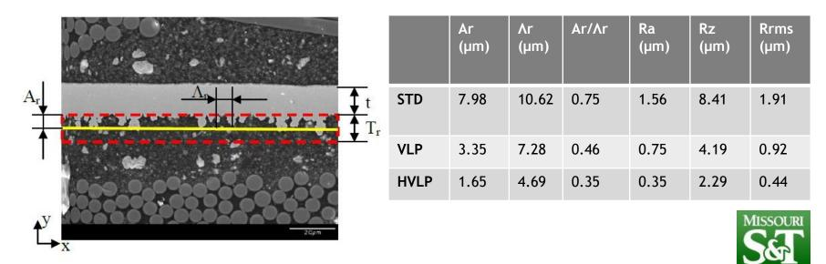
Fig. 6. Magnified section of the signal trace conductor in the SEM picture of the test line with STD foil. The region of the "roughness dielectric" is selected by a dashed line
