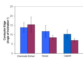
Surface Finish Thick film printed circuit have very sharp edges 7-15 degrees. Results shown for 2 types of silver paste on 3 surfaces
