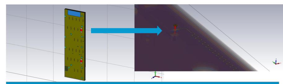
Materials properties Dielectric: eps=3.6, tgd=0.01 Debye 3<sup>rd</sup> order Copper = 4.1e7 S/m with inclusion of surface roughness with TSI (H&J model)
