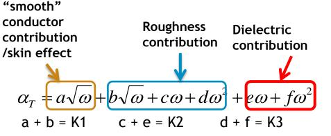
•Curve fitting co-efficients are generated K1 ~  $\int \omega$ , K2 ~  $\omega$ , and K3 ~  $\omega^2$
