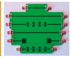
**1(c)** Extracts DUT S-parameters using just Thru and Line calibration standards\*.
