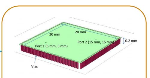
Fig. 5. Geometry of the shorted resonator simulated using Sonnet and the rapid plane solver.
