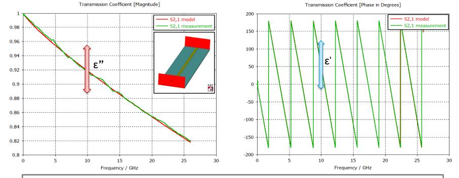
The measured  $S_{21}$  of homogeneous transmission line section is used for an extraction of substrate complex permittivity. Please note that transmission coefficient  $S_{21}$  is equal to  $exp(-\Gamma L)$  or "egL", where Gamma is the propagation constant and L is the length of TL.
