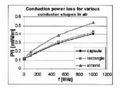
Power loss results comparing "Almond" and "Rectangle" shape with same cross-sectional area. Larger loss with "Almond" shape @ 1GHz, difference of ~38% conductor loss
