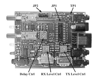
Figure 4 ó Location of TP1, JP1, JP2 and the TX, RX, and Level controls.
