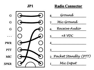
Figure 3 ó Example Jumper Wire Diagram for TS-450
