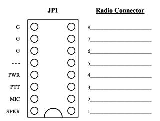
Figure 2 ó Jumper Wiring Diagram
