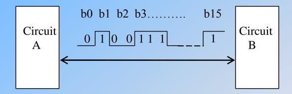
Sending a byte or a word in parallel, sequentially (commonly used between circuits within a computer)
