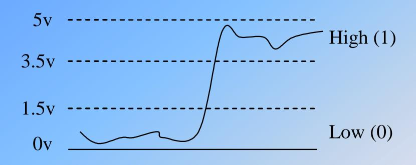
Digital Signal has <u>a high noise immunity level</u> the level of noise that can be added to the signal without affecting its state.
