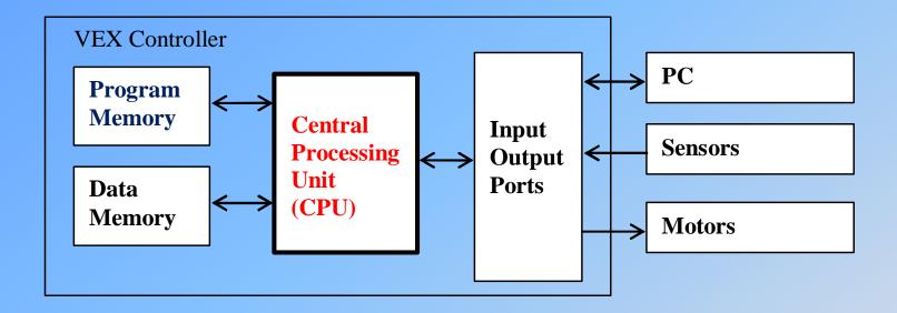
CPU: Executing instructions, performing arithmetic and logic operations. It is the 'brain' of the computer.Memory: Memory is for keeping program and data.
