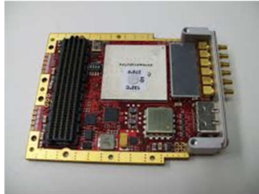
Parallel e2v EV10AQ190 10-bit chip on card
