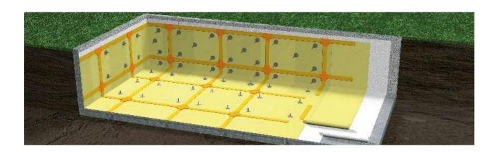
A compartmental waterstopping system composed of **Sika® Waterbar** and welded single or double layer **Sikaplan®** sheet membranes is combined with Sika injectable pipes and ports casted into the concrete structure, to provide the security of complete watertightness control,
