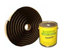
**Lockstop** is a single component and self-sealing mastic waterstop which bonds to concrete to prevent moisture from penetrating nonmoving joints. Lockstop must be used in conjunction with **Lockstop Primer Adhesive** to create a watertight bond.
