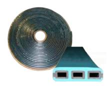
**Hydrotite** is a world renowned hydrophilic waterstop. Composed of modified chloroprene rubber protected with a special delay coating, Hydrotite expands when exposed to water, creating an effective compression seal within joints where limited movement will occur.
