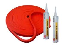
SikaSwell®-A (formerly Duroseal Gasket) is a water-swelling acrylate-ester that expands upon contact with water to form a compression seal in nonmoving concrete joints. SikaSwell®-A is a available in three sizes and is adhered to varying substrates with Sika® MK Adhesive or Quellpaste Type E.
