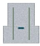
Strip-applied Waterstops are adhered along concrete joints or penetrations and encapsulated by a subsequent concrete placement. Hydrotite is the state of the art for hydrophilic waterstop and is a high-performance, chloroprene rubber material that expands when exposed to moisture to create a compression seal within and along the joint. For less critical applications, Sika also offers SikaSwell®-A and Sika® Swellstop® expanding waterstops.
