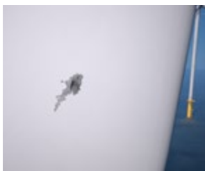
Structural composite damage.
