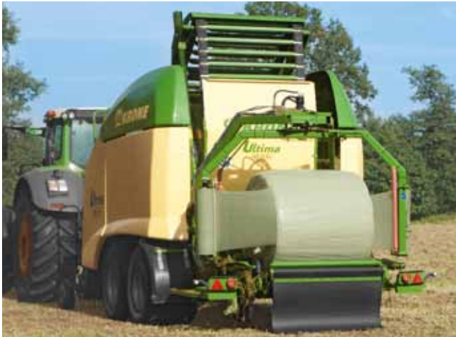
Film pre-stretch should be up to 70 %
