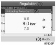
The upper and lower limit of the setting is shown in grey, the actual setting is shown in black. Use the  $\uparrow$  or  $\downarrow$  key of the Scroll keys to modify the settings as required and press the Enter key to accept.
