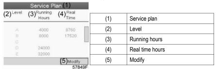
In the example above, the A Service level is programmed at 4000 running hours, of which 0 hours have passed. History
