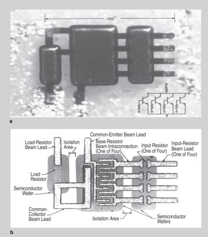
Figure 2. The top and bottom view of a four-input DCTL gate.<sup>2</sup>
