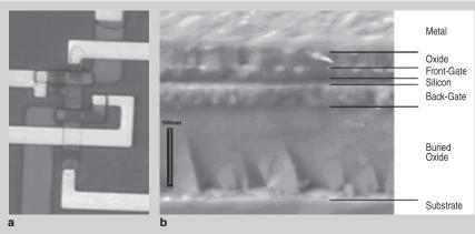
Figure 6. (a) An optical microscope photograph of a signal inverter circuit fabricated with a silicon crystal layer of nanoscale thickness and with control gate electrodes fabricated both above and below the active silicon layer. (b) A scanning electron microscope image of the silicon wafer from which the circuit shown in (a) is fabricated. The electronically active part of the structure is the thin silicon layer sandwiched between the back-gate and front-gate layers in the image.<sup>16</sup>
