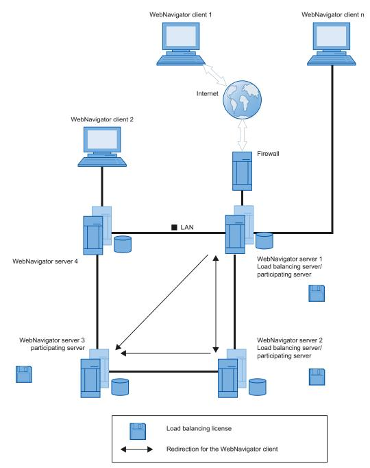
In the figure, WebNavigator Servers 1 to 3 participate in "Load Balancing". A "Load Balancing" license is installed on the WebNavigator Servers.
