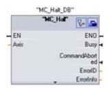
MC\_Halt cancels all motion processes and causes the axis motion to stop. The stop position is not defined.
