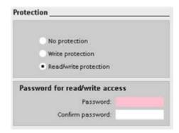
Each level allows certain functions to be accessible without a password. The default condition for the CPU is to have no restriction and no password-protection. To restrict access to a CPU, you configure the properties of the CPU and enter the password.
