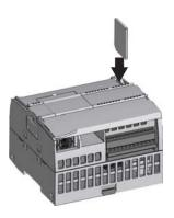
To insert a memory card, open the top CPU door and insert the memory card in the slot. A push-push type connector allows for easy insertion and removal. The memory card is keyed for proper installation.
