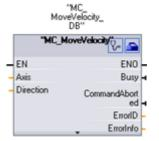
MC\_MoveVelocity causes the axis to travel with the specified speed.
