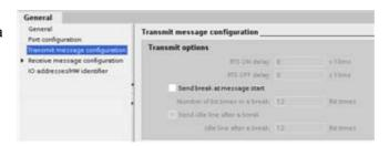
You can also dynamically configure or change the transmit message parameters from the user program by using the SEND\_CFG (Page 254) instruction.
