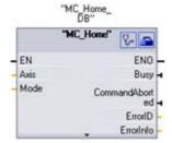
MC\_Home establishes the relationship between the axis control program and the axis mechanical positioning system.
