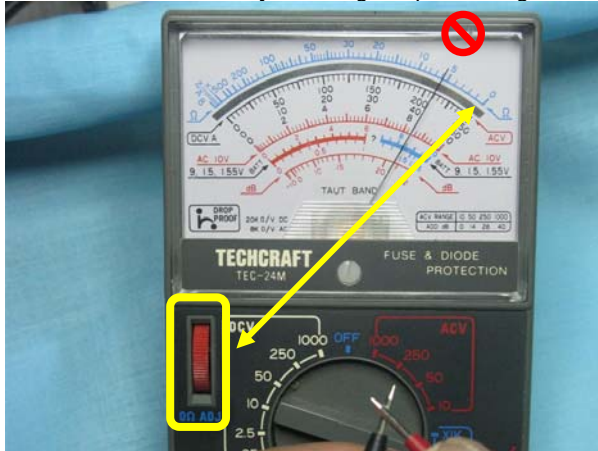
If it is not "0 Ω" use the "0 Ω Adj" knob to adjust the needle to read "0 Ω"
