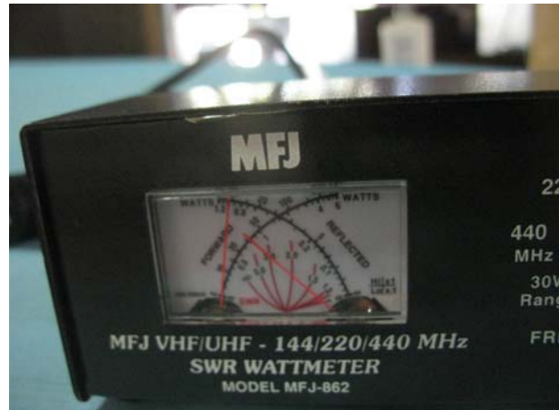
The SWR is off the scale indicating a problem with the coax being tested.
