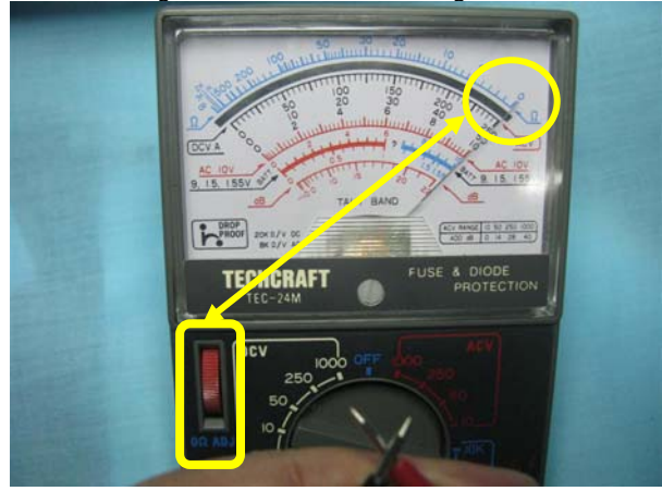
If it is not "0 Ω" use the "0 Ω Adj" knob to adjust the needle to read "0 Ω"
