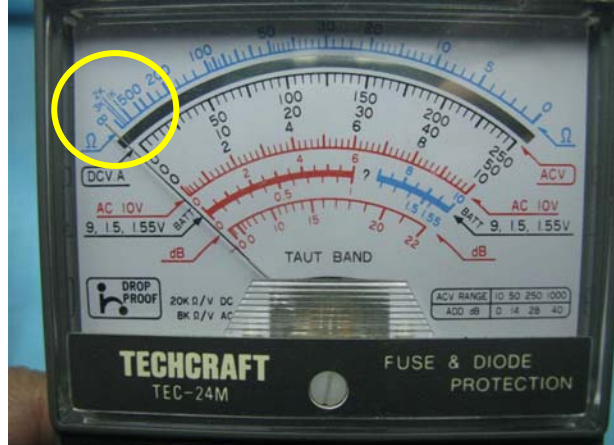
A high reading on the \Omega scale means there is no conductivity between the shell and the center pin.
