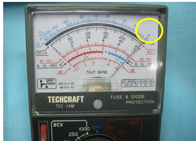
The reading shows "0 \Omega " meaning no resistance; there is a short in this assembly.
