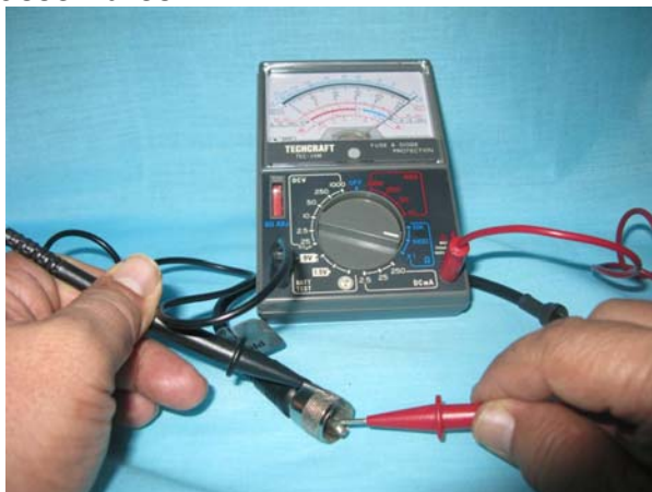
Test leads are on Shell 1 and Pin 1.
