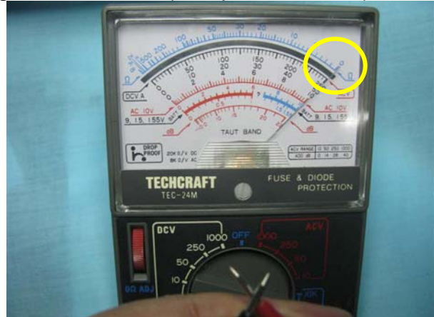
The reading should be "0 \Omega " meaning no resistance.
