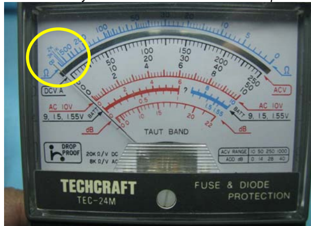
So far, so good. There should be no electrical conductivity between the shell and the center pin.
