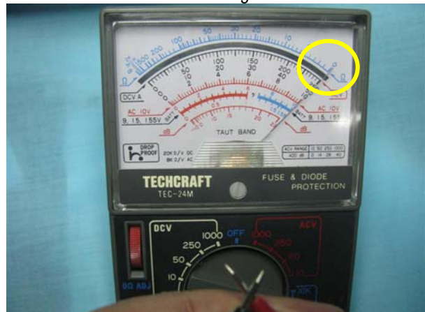
The reading should be "0 Ω" meaning no resistance.
