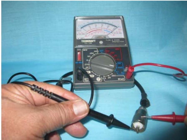
Test leads are on Pin 2 to Shell 2
