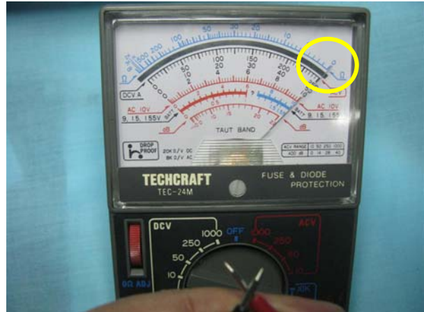
The reading shows "0 Ω" meaning no resistance.
