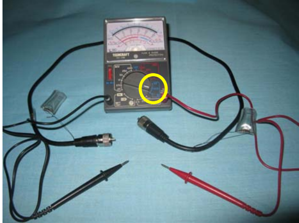
Turn the selector to "Ω" to measure continuity.
