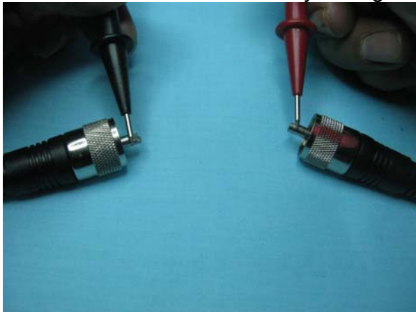
Put a test lead on each center pin and check the reading.
