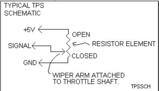
You can determine the connections of the factory TPS using the following information: The TPS should be in a closed throttle position.
