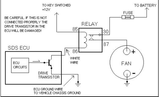
Fuse rating will depend on the current draw of the fan(s). 15 Amp may be fine for most applications. If two fans are used a 20 Amp fuse may be needed.
