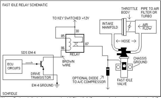
\*Note: Optional diode is not required if Pin 13 A/C sense wire is connected to the A/C clutch positive wire. Only use diode on "D" (fuel only) type SDS systems.
