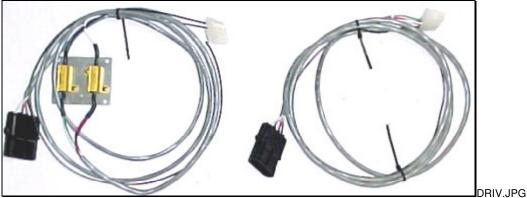
The injector drive harness has a white plastic plug that connects out to the injector harness as well as optional relays or optional knock sensor. The system comes with one of the above harnesses. Left shows low impedance drive harness with resistors. Right shows high impedance drive harness which has no resistors. (4 cylinder shown).
