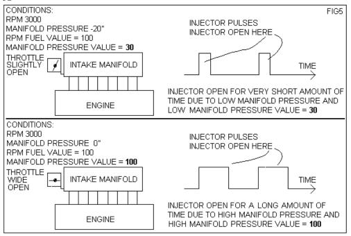
Use gauge1 mode to see what manifold pressure range the engine is running in, then use the < > keys on the programmer to move to the range you want, then you can try adjusting the values if desired. Below we will explain different areas of tuning MAP sensor values. These are divided into sections, idle, part throttle, full throttle/low boost, high boost, deceleration.
