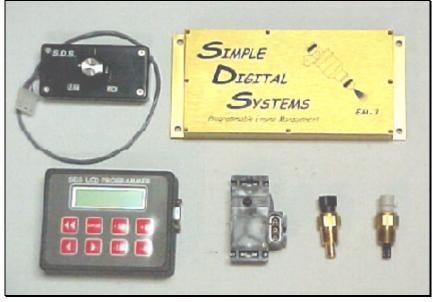
Top left Mixture knob. Top right SDS ECU. Bottom left: SDS Programmer. Bottom middle MAP sensor. Bottom right Engine temp and Air temp sensors.
