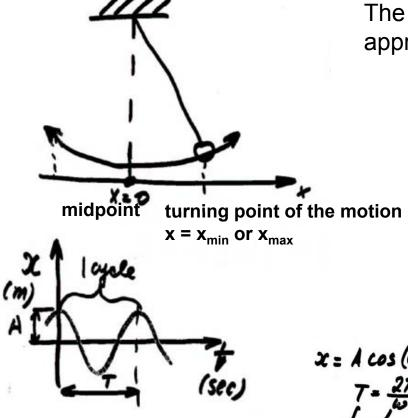
The motion of a pendulum is approximately simple harmonic
