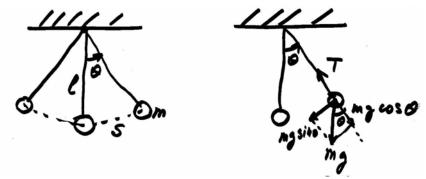
**Restoring force = -mgsin0** Apply  $2^{nd}$  Newton's Law: F = ma =>  $-mgsin\theta = ma =>$
