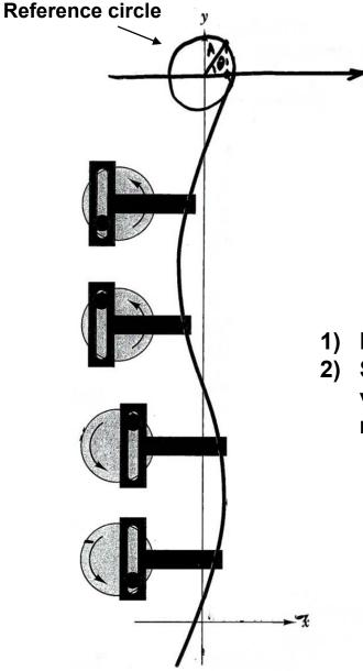
Simple mechanism for generating simple harmonic motion from uniform circular motion.
