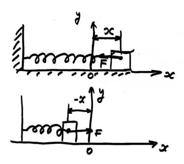
After positive displacement of the mass the spring pulls the mass back toward the equilibrium position – the relaxed length of the spring.
