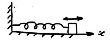
The motion of a mass oscillating back and forth in response to the push and pull of a spring – simple harmonic
