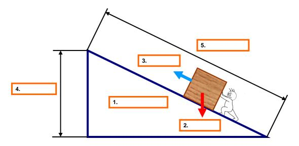
**2.** A person wants to build an inclined plane to move a box to a higher lever. The height he wants to reach is 3 m. The mass of the box is 85 kg and he is able to push with a 500 N force. Work out the needed length of the ramp and the mechanical advantage of the inclined plane.
