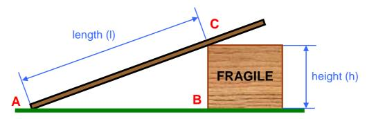
**b)** Measure the length (I) and the height (h) of the plane with a measuring tape.
