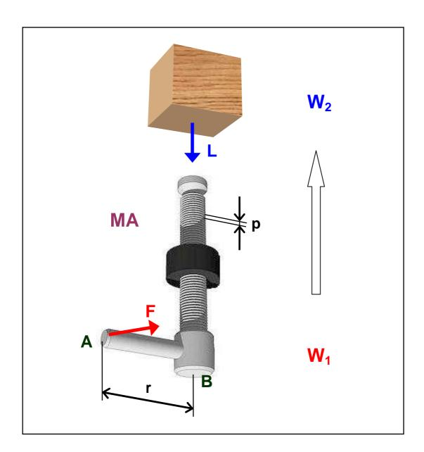
**a)** Measure the length (r) of the handle (the distance from A to B) using a ruler, a measuring tape or a calliper.
