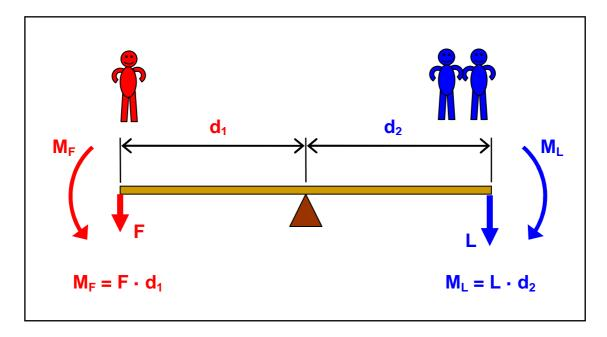
Multiply force F by its arm  $d_1$  and you will get the moment of force  $(M_F)$ . Multiply load L by its arm  $d_2$  and you will get the moment of load  $(M_L)$ .
