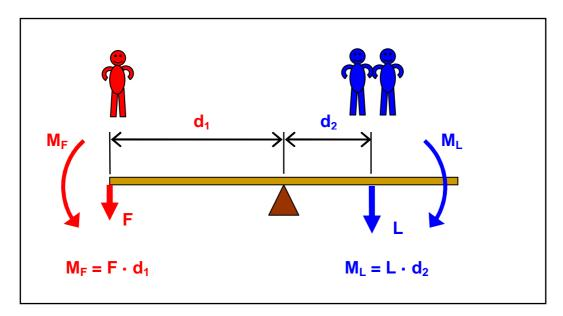
*j)* Work out the mechanical advantage of the seesaw with the new distance  $d_2$ .
