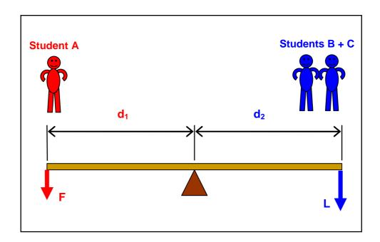
**d)** Using the measuring tape, measure the distance between both seats and the centre of the seesaw. These distances will be the force arm ( $\mathbf{d_1}$ ) and the load arm ( $\mathbf{d_2}$ ).
