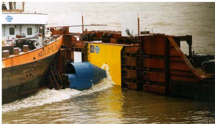
Figure 2-2: Full-scale collision experiment in the Netherlands (Wevers et al 1999).
