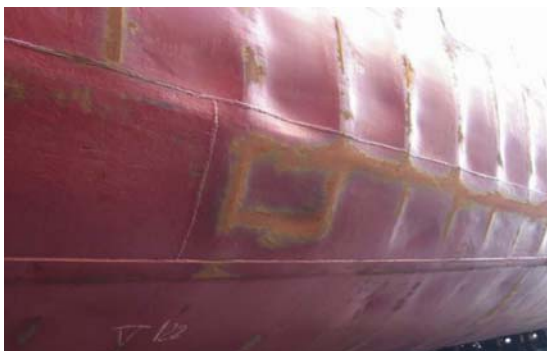
Figure 4-3: Side plating damage of ships navigating in ice (Hänninen 2003).
