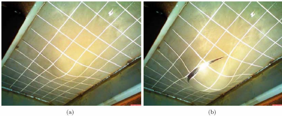
Figure 2-6: Indentation of a bare plate (a) before fracture, (b) after fracture (Alsos and Amdahl 2008).
