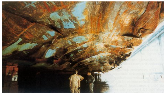
(b) El Paso Paul Kayser – an LNG carrier in dry dock after grounding in Straits of Gibraltar (Photo Courtesy of BP).
