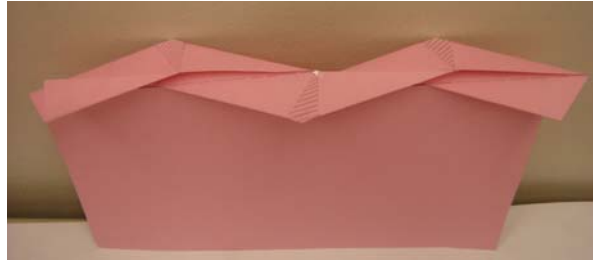
Figure 3-14: Sliding deformation model for web girders during sliding reproduced from paper folding.
