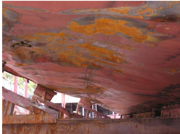
(a) Bottom damage of MS Sveafjell ran aground on the coast close to Trondheim, Norway (Photo Courtesy of Alsos, H.S.).
