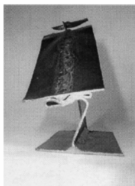
Figure 3-5: Cross-section profile of web girder after crushing test at DTU (Simonsen and Ocakli 1999).
