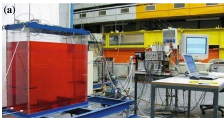
Figure 1: The scaled-down tank model on the shake-table [7]
