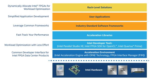
Figure 1. Acceleration Stack for Intel Xeon CPUs with FPGAs
