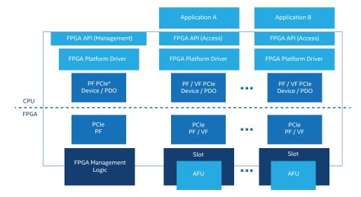
Figure 3. FPGA Driver
