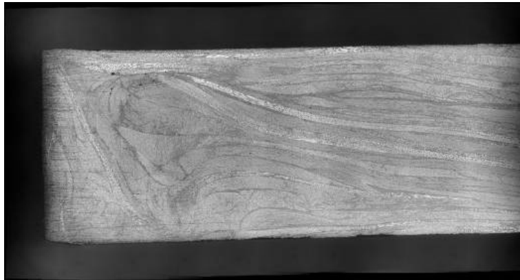
Figure 5: Optical micrograph of edge of plate region showing nonplanar chip formation, specimen 6R
