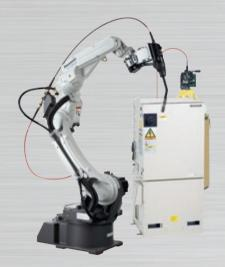
The new Super Active torch with air cooling mechanism increases the duty cycle and allows use in higher current ranges.
