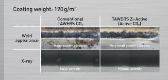
Between 75% – 95% of the spatter reduction compared to
