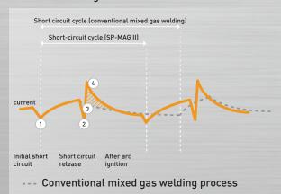
A stable short-circuit sequence is achieved by the superimposition of the waveform.
