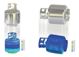
FIGURE 6: PROPANE TANKS DROPPED IN DIFFERENT ORIENTATIONS SHOW SIGNIFICANTLY DIFFERENT STRESS RESULTS.
