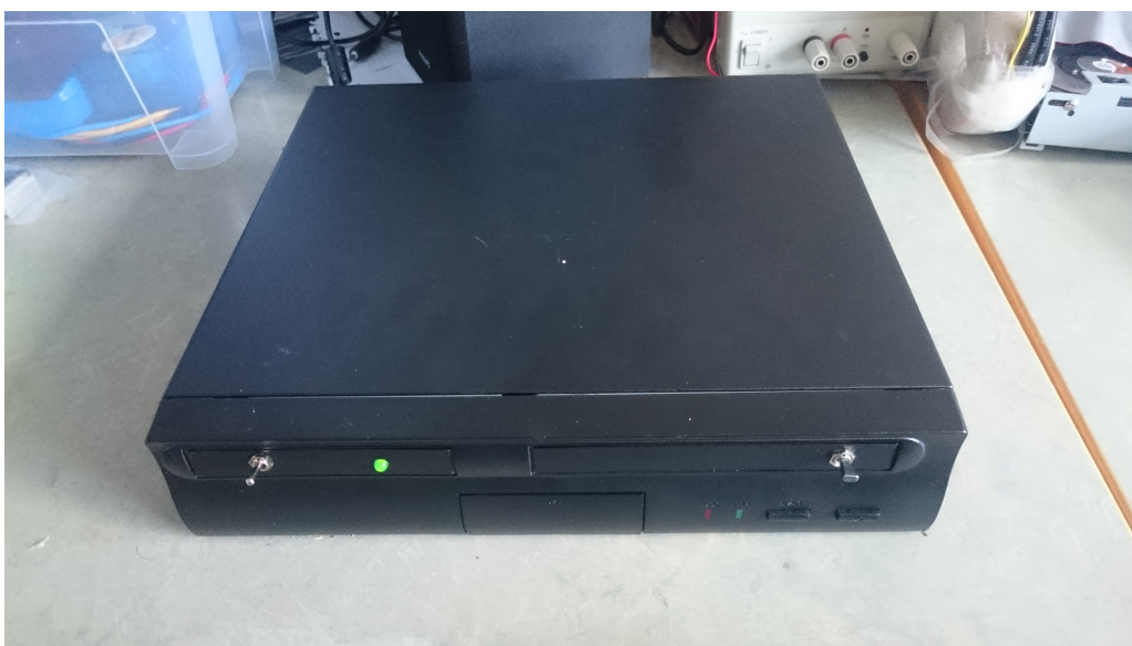
Figure 6: The chassis in which the PCB was mounted, with a power switch and a standby switch.
