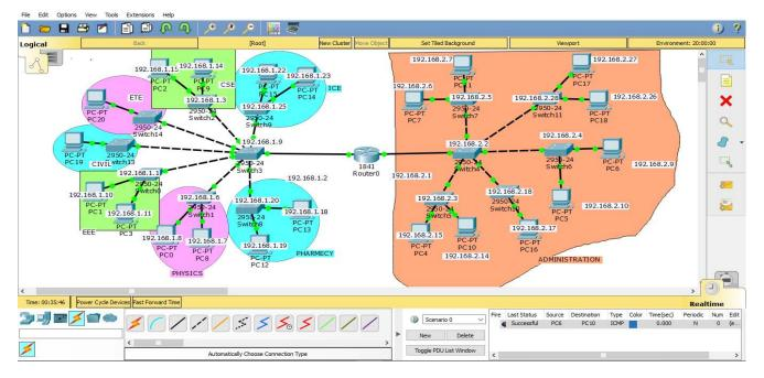
Fig. 3: The complete diagram of University Area Network Scenario created in Packet Tracer environment
