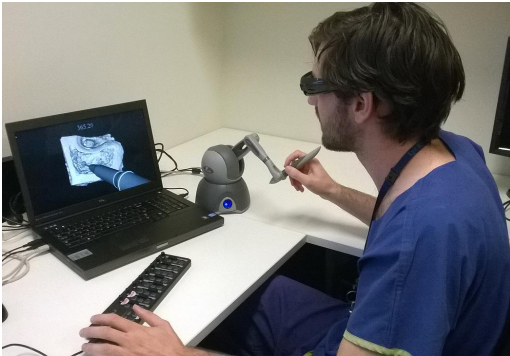
Figure 1: The University of Melbourne VR temporal bone surgery simulator.
