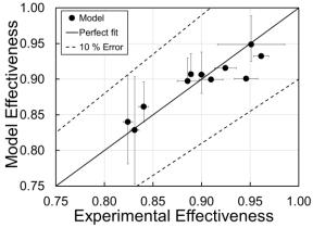
Figure 2. Model predicted vs. experimentally measured effectiveness.
