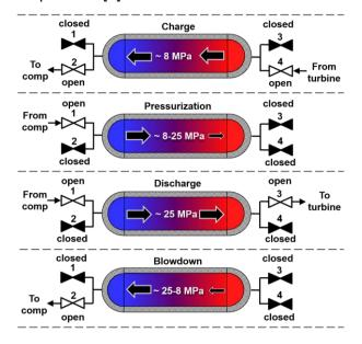
Figure 1. Regenerator operating processes.
