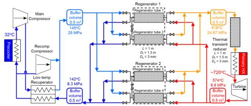
Figure 5. Schematic of the high-temperature regenerator in a Brayton recompression cycle.
