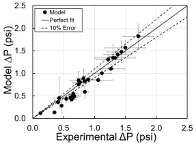
Figure 3. Model predicted vs. experimentally measured pressure drop.
