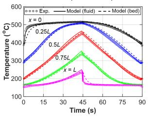
Figure 4. Model predicted vs. experimentally measured regenerator temperature profiles.
