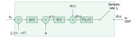
Figure: Baseband Equivalent System to be Simulated.
