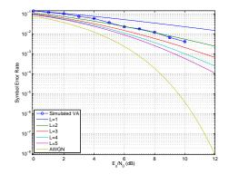
Figure: Symbol Error Rate with Viterbi Equalizer over Multi-path Fading Channel; Rayleigh channels with transmitter diversity shown for comparison. Baud rate 1MHz, Delay spread  $\approx 2\mu$ s.
