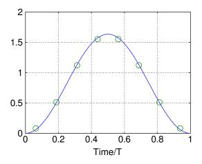
Figure: Discrete-time Equivalent Impulse Response ( $f_s T = 8$ )
