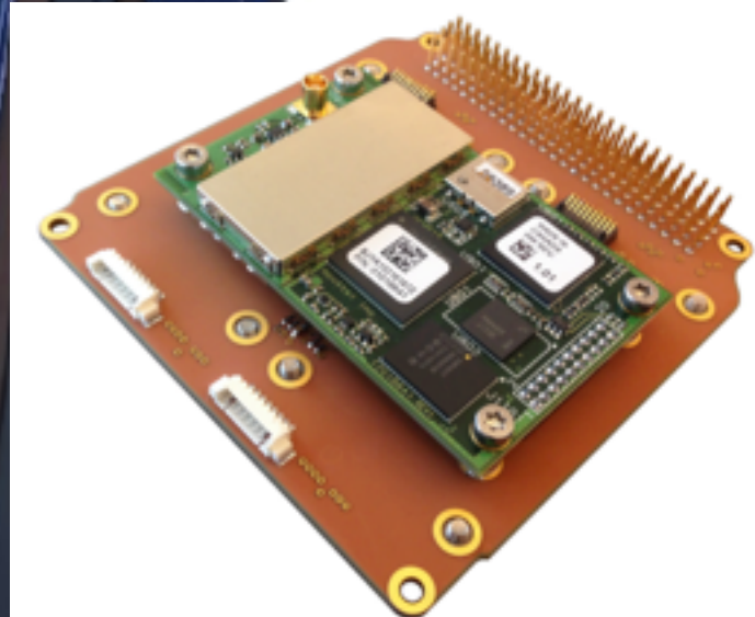
GPS mounted to Motherboard
