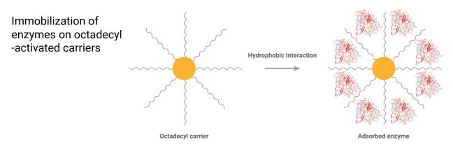
Lifetech<sup>™</sup> ECR1090M and ECR1030M have a high degree of hydrophobicity due to the presence of styrene and divinylbenzene (DVB). These resins are optimal for the immobilization of lipases, are stable during storage and can easily be handled before and after immobilization procedures (Figure 8).
