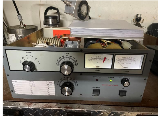
The Command HF-2500 amplifier undergoing initial tests after installing 4 new LED meter bulbs. The 3-ring binder is holding down the interlock switch.
