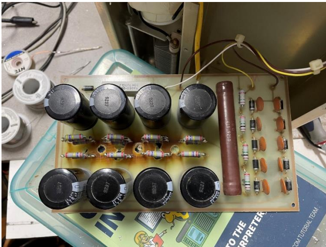
The power supply PCB. Note the burn marks from the capacitor equalization resistors.
