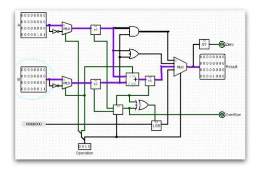
Make sure you understand how the Operation 4-bit input is used to control the function of the ALU.
