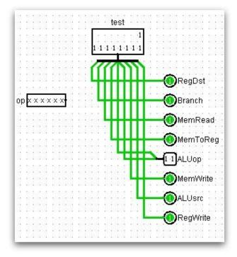
NOTE: All output lines from the control unit but the ALUop are 1 bits.
