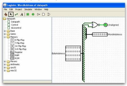
This is a small sub circuit used to translate a 32 bit address to a 8 bit word address.
