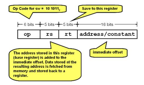
For this instruction the ALU is used to calculate the final memory address.
