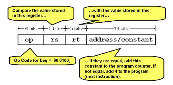
To compare the two registers the ALU can be used. For two number A and B, A-B == 0 IFF A == B.
