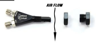
recommended nozzle location will be mounted into the inlet tube 2-6" in front of the throttle body. On a single nozzle dry system the nozzle will be placed in the air box before the mass air meter. Certain custom applications will dictate other nozzle location.
