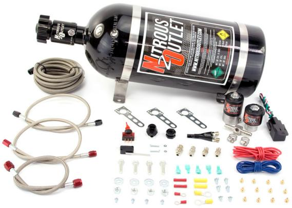
Your system should come with everything you see here, the fuel feed/adapter fitting may vary for vehicle specific systems. You will have everything you need to install a nitrous system on your vehicle; main feed line, fuel adapter fitting, nitrous and fuel lines, solenoids and brackets, electrical fittings and wire, relay and harness, bottle brackets, wide open throttle switch, toggle switch for system arm, nozzle and nozzle adapter, jetting for up to 200HP.
