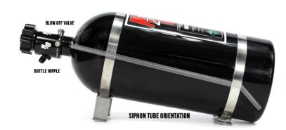
If mounting the bottle vertically, the valve handle and label must face toward the front of the vehicle. This position will orientate the siphon tube at the back of the bottle where the liquid nitrous will be during acceleration.
