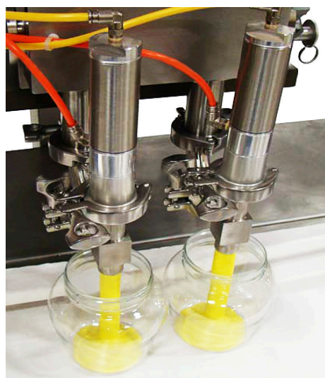
Above: Hand depositing nozzle filling cups with apple pie filling. Below: 1" vertical cut-off spouts filling jars with mustard.
