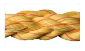
Our range of floating pick-up / messenger lines are based on Lankhorst TIPTO® brand ropes. These ropes exhibit high strength, excellent abrasion resistance and energy absorption properties, ensuring a long service life. The low weight makes messenger line handling on board easier. Lankhorst TIPTO® brand ropes are supplied in high visibility yellow colour and have a specific gravity of 0.93 – self floating.
