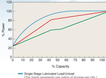
Single-Stage Lubricated Load/Unload
