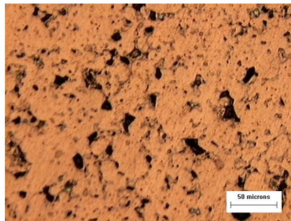
Figure 11. Optical micrograph of the ternary alloy Cu-0.5%Ni-0.5%Cr, cold compact (20MPa) and sintered at 1053K for 5.4 \times 10^3 s and also homogenized at 773K for 32.4 \times 10^3 s.
