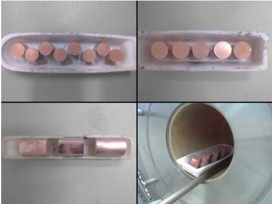
Figure 1. Ternary Cu-Ni alloys distributed in alumina boat for sintering and homogenizing heat treatment in vacuum furnace.
