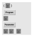
By pressing the <Area switchover key> ( ) repeatedly, you are able to go back and forth between the two operating areas last active what is quite useful, e.g. when programming to see the tool data in parallel.
