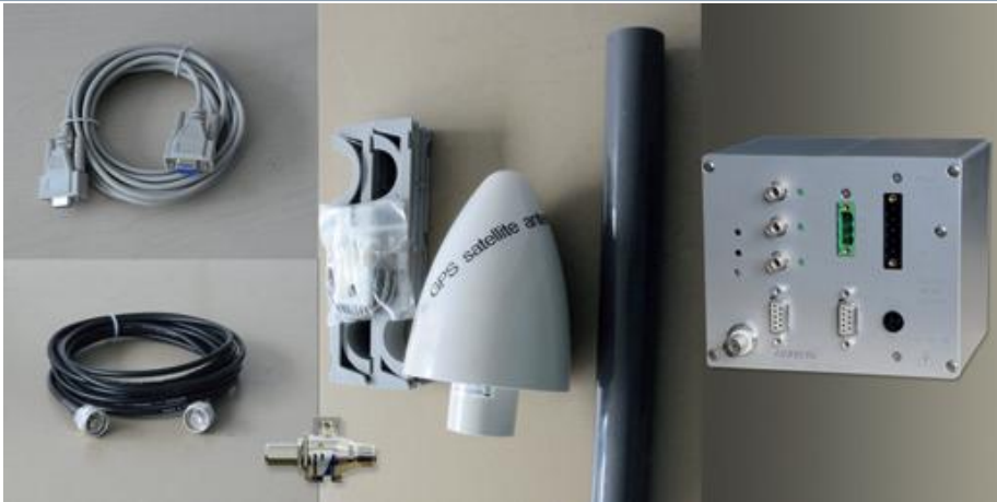
Fig. 14 GPS Time Synchronization Unit 7XV5664-1AA00 contains of: 1 x Parameterization Cabel (left above), 2 x Communication cable (50m +5m RG58) Antenna -> Lightning protection -> GPS Receiver (left below), Lightning protection (below), Antenna with mounting kit (center), GPS Receiver (right)
