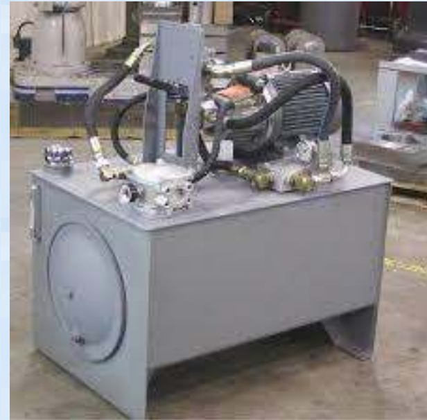
Power Pack AC motor, pompa, reservoir Relief valve
