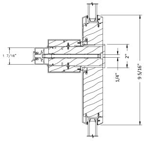
VERTICAL MULL SECTION TRANSOM OVER WIDE STILE UNIT WITH 1/4" REINFORCEMENT
