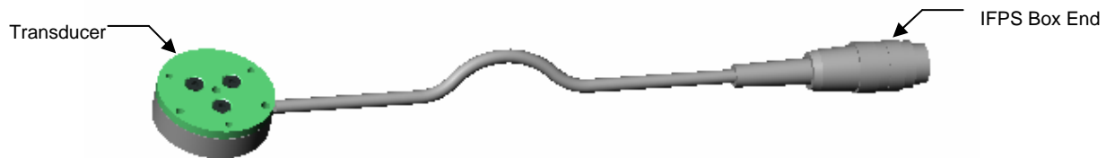
Figure 2.2b—Integral Transducer Cable on Small Transducers
