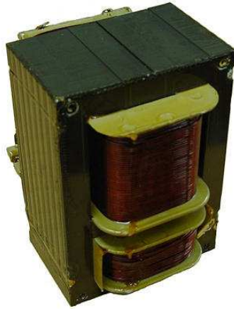
Figure 9.10: Example of a gas-discharge lighting transformer.
