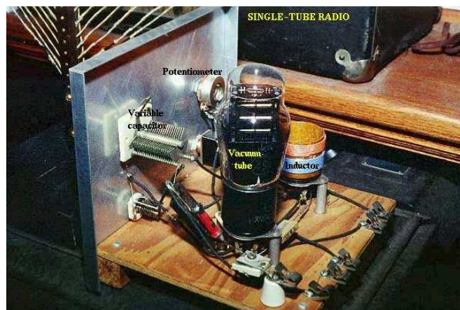
Figure 8.24: Variable capacitor tunes radio receiver tank circuit to select one out of many broadcast stations.
