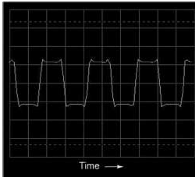
Figure 7.31: Oscilloscope time-domain display of a square wave
