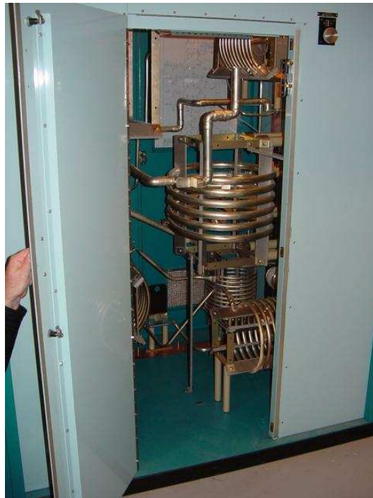
Figure 3.18: High power inductors formed from hollow tubes.
