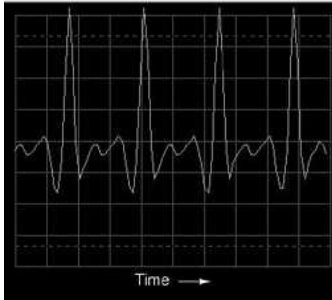
Figure 7.27: Oscilloscope display: waveshape of a trumpet tone.
