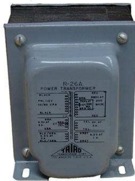
Figure 9.30: Photograph of multiple-winding transformer with six windings, a primary and five secondaries.
