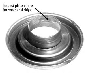
PLEASE: Don't hone, sand, scrape, polish or try to fix the piston in anyway. Leave it as-is. If it's really bad, replace it and use the new expander & seal for a long term fix.
