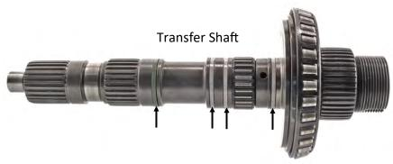
These 4 rings like to shrink dumping lube oil that can lower main line and accelerate ring land wear on the low clutch housing. 68018615AA
