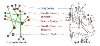
Figure 7: Four different types of hydraulic nodes.
