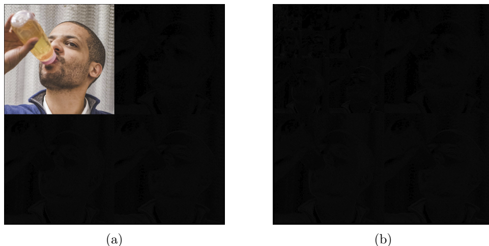
Figure 7.1: The original image was 2048x2048 pixels. Image (a) applies just one level of the 2D Haar Wavelet Transform on each of the RGB values per pixel separately, and (b) applies the full recursion down to the 1x1 base case. The resulting image is approximately sparse (RGB values of (0,0,0) correspond to black). If one zooms into this document and looks closely, some object edges are still visible after the transform (the outline of my head and jacket collar), albeit faintly.
