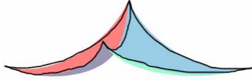
Fig. 13. Result of reconstructing the symmetrically curved surfaces. The sketch is the set of solid dark lines while the recovered curved surfaces are color-coded.
