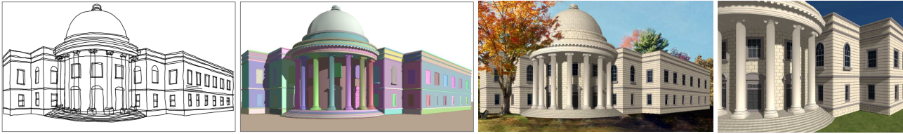
Fig. 1. Sketching reality example (rotunda), from left to right: Sketch of building, extracted 2.5D version, rendered model with a new background and rendered result with different view and lighting.
