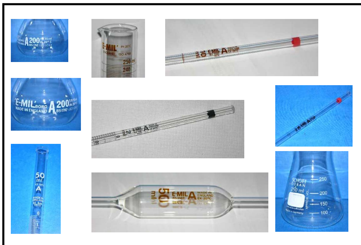
Figure A3.8: Illustrations of markings on volumetric glassware
