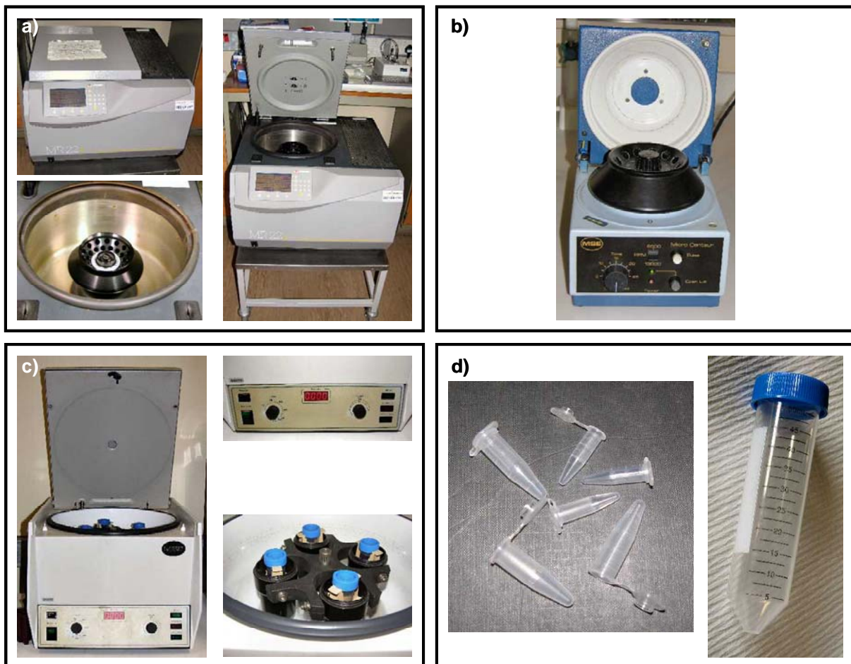
Figure A3.19: Different types of centrifuge, (a) to (c), and centrifuge tubes (d)
